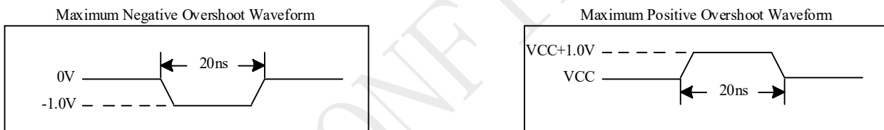
Figure 5-3 Maximum Overshoot Waveform
